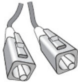
A sample LC fiber-optic connector
